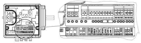
Fig. D-2 Electrical connection diagram of frequency converter
