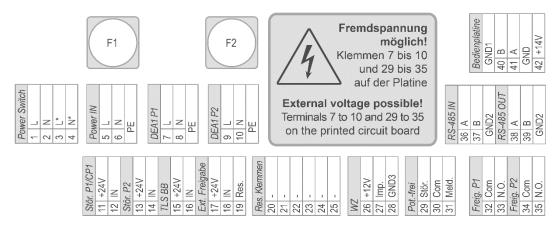
Fig. D-2 Connection diagram for the pressure booster system control unit
