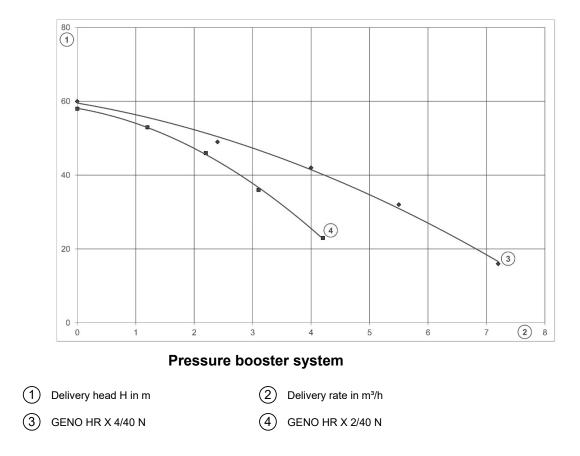
Fig. C-5: Centrifugal pump characteristic curve GENO-HR-X 2/40, GENO-HR-X 4/40
