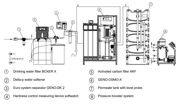
Fig. D-1: Installation example for pressure booster system GENO-FU-X
