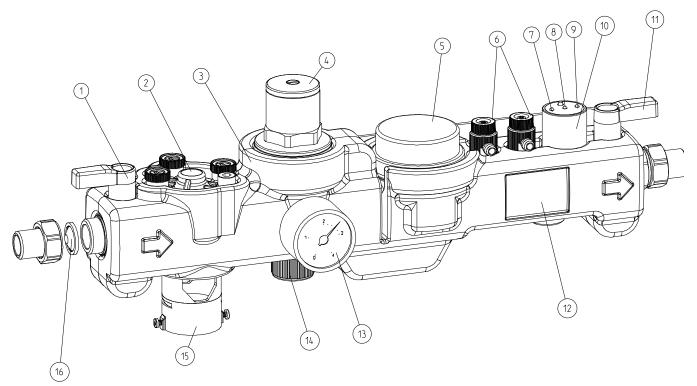
Fig. C-2: Position drawing of GENO-therm® filling device Komfort
