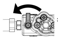
3. Slowly open the shut-off valve (inlet) upstream of the filling device. The filling device then moves into the operating position.
