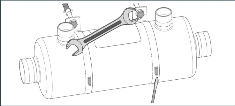
5. Insert the heat exchanger.
