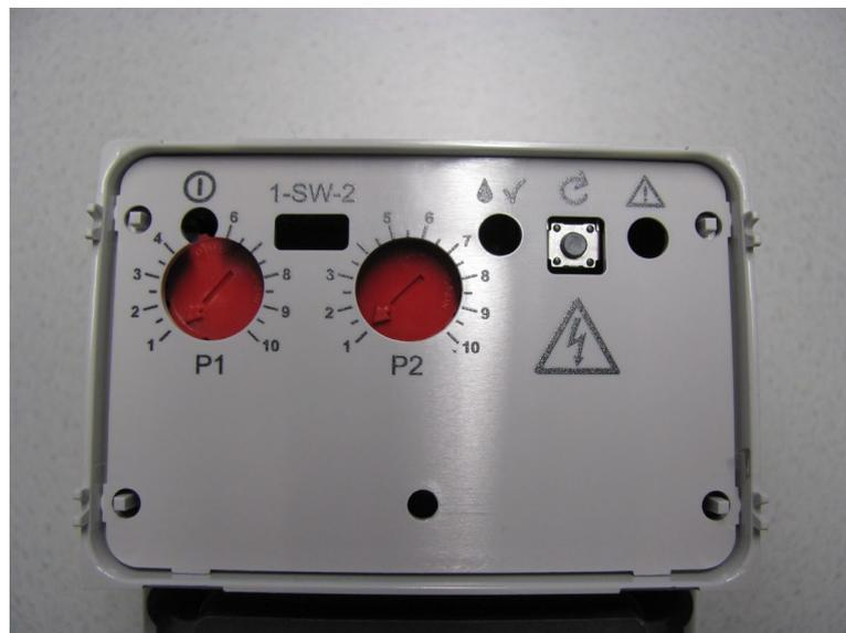
Fig. E-1: Potentiometer coarse (P1) and fine (P2)
