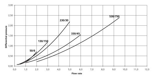
Fig. D-2: Pressure loss curve for GENO-mat® duo WE
