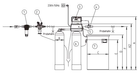
Fig. D-1 (a): Installation drawing for water softener GENO-mat®-duo WE
