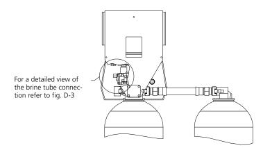
Fig. D-2: Water softener GENO-mat®-duo WE; rear view
