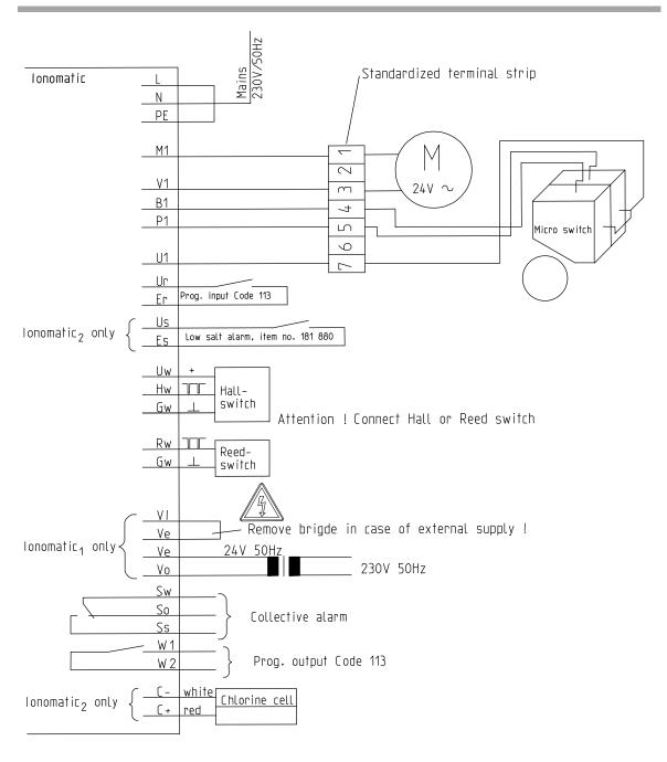
Fig. D-2: Terminal plan
