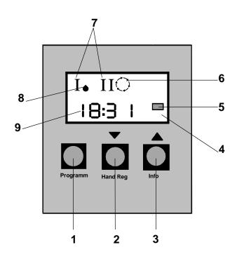
Fig. F-2: GENO®-IONO-matic controller; operational controls and display
