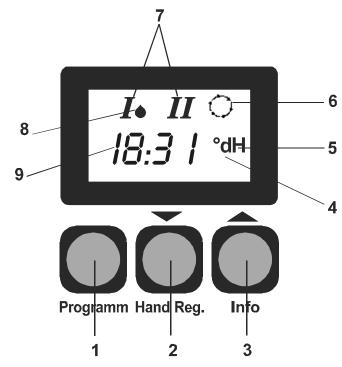
Fig. F-2: Control unit GENO-IONO-matic; operating elements and display
