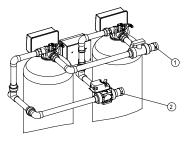
Fig. C-7: Piping with three-way ball valve with actuator
