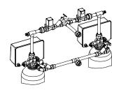
d) Solenoid valves (nominal connection widths DN 20 and DN 25)
