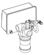
Fig. C-2: Control valve Nominal connection width DN 40
