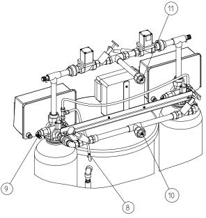
Fig. D-6 (b): Water softener GENO-mat-duo WF, rear view
