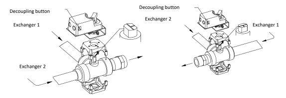
Fig. D-3: actuator with 3-way-ball valve; backside view
