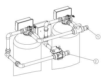
Fig. D-2: Example for the piping of medium-sized and large systems; no actuator for large systems.
