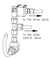
Fig. C-5: Disinfection device (pre-assembled)
