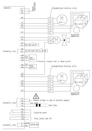
Fig. D-9: Terminal plan for medium-sized systems (nominal connection width 1½")
