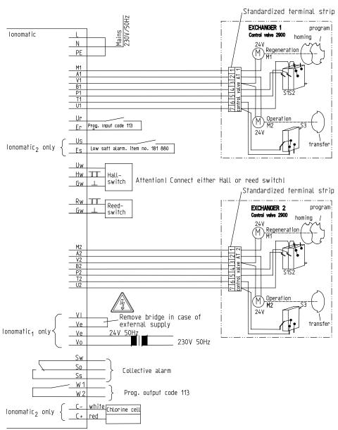
Fig. D-10: Terminal plan for large systems (nominal connection width 2")
