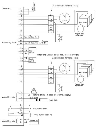
Fig. D-7: Terminal plan for small systems (nominal connection widths 3/4" and 1")
