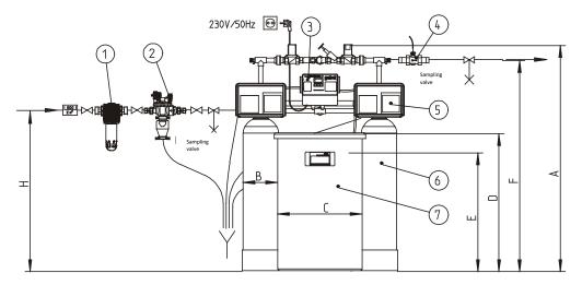
Fig. D-6 (a): Installation drawing for water softener GENO-mat duo WF
