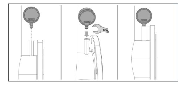
1. Screw the pressure gauges to the flanges at the top of the support pipe.
