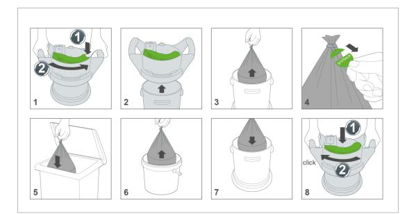
If the resin bags need to be replaced during a treatment process (connected mixed bed cartridge), please take the following into account:
