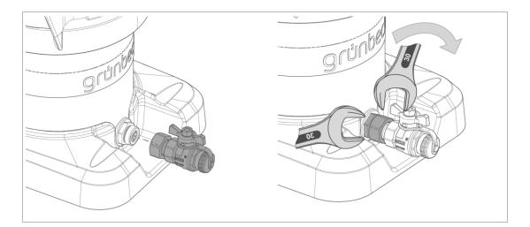
Install the shut-off valve - with the seal being inserted - on the raw water connection (inlet) of the mixed bed cartridge.
