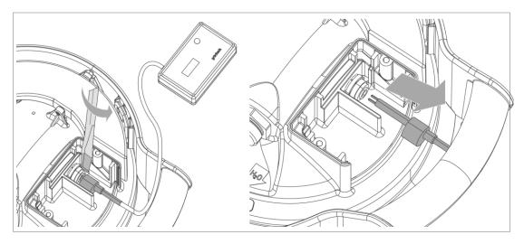
**4.** Press the retaining ring of the quick connector (using a flat-head screwdriver) and at the same time carefully pull out the conductivity sensor.
