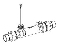
Fig. 3: Turbine flow mete Softener version
