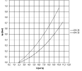
Fig. 2: Pressure loss curve TWZ
