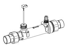
Fig. 2: Turbine flow meter EXADOS version
