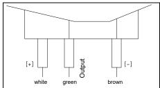
Fig. 3: Terminal plan
